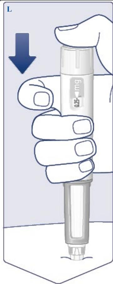
**Press and hold down the dose button until the dose counter shows  $\text{•}0\text{•}$ .**
